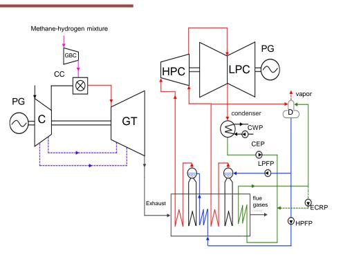
An increase of the H2 concentration to 30 vol. % leads to CO2 emission reduce in the flue gasses by 15%.
