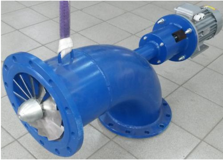
Figure 7. Photograph of the hydraulic unit model with a propeller turbine.
