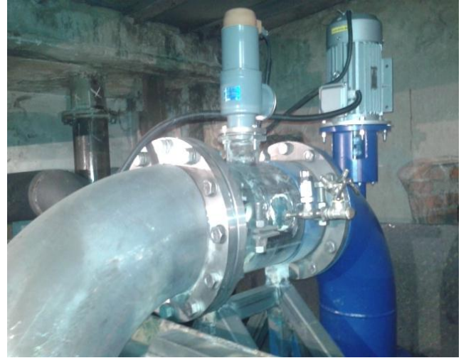
Figure 8. Photograph of the siphon penstock model fragment of the micro-HPP on the experimental bench.
